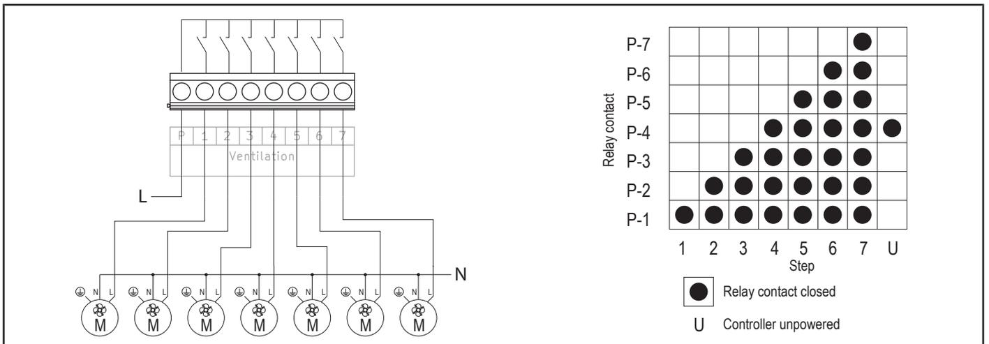
Illustration 3: ETD-CN Step contacts wiring diagram
