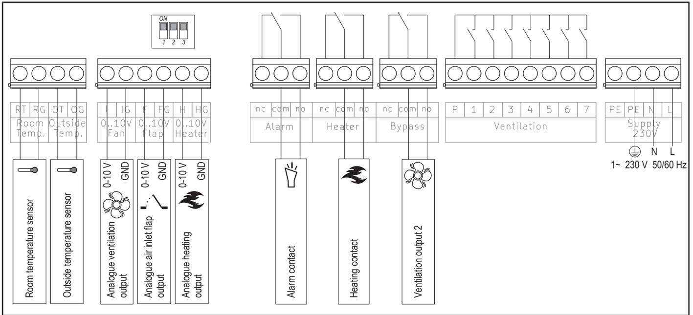
Illustration 1: ETD-CN Main wiring diagram
