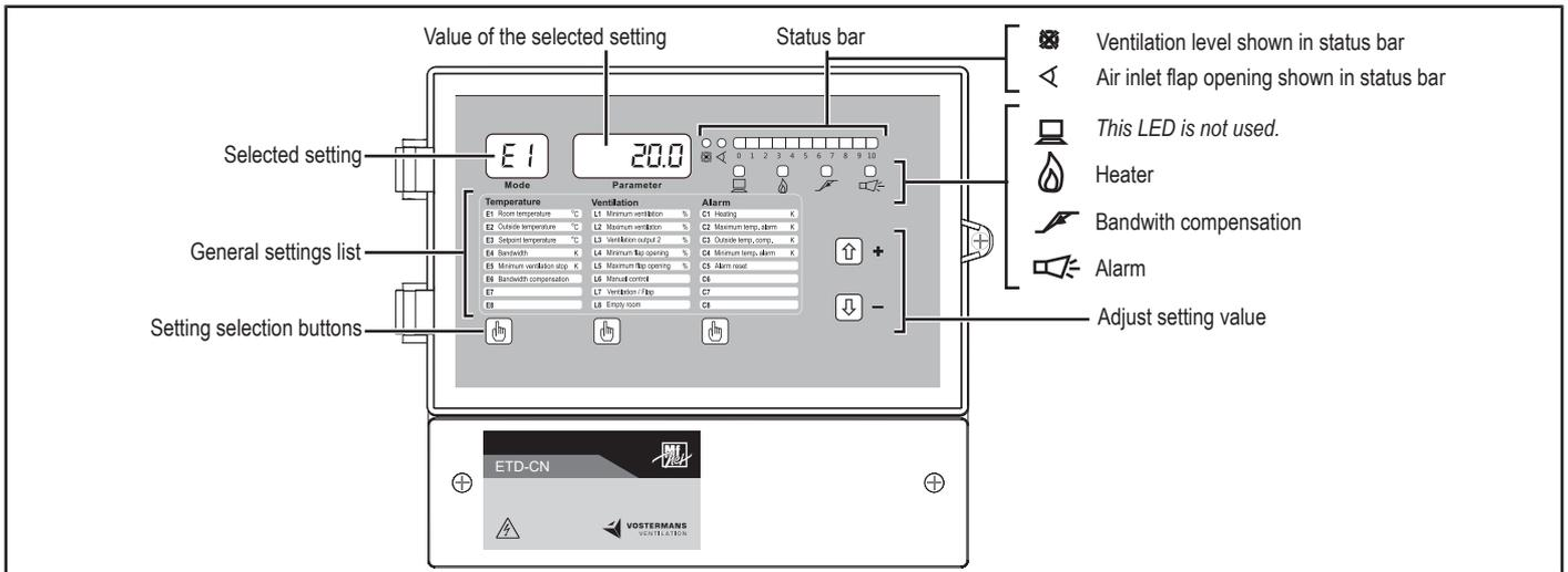
The settings list on the controller is default in English. Labels to change the settings list to Dutch, German or French are included with the controller. The controller display language is English and this cannot be changed.
